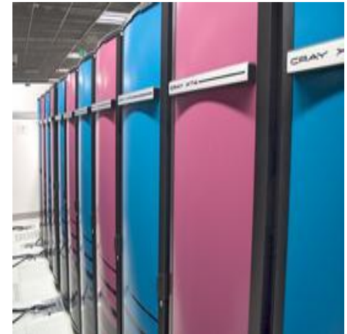
Louhi: Cray XT4/XT5 with 2.3 GHz 4-core AMD Opteron. All-in-all 9424 cores and Peak power of 86.7 Tflops.
